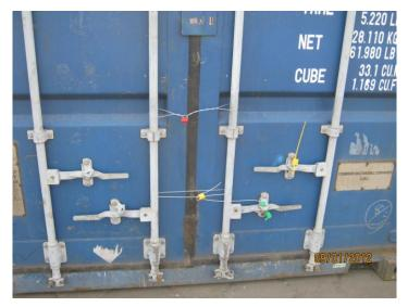
One such preventative measure is to bind the container doors using wires and seals. Taking pictures of the container doors will also help to assist defending any claim the ship may be presented with.
