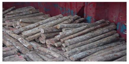
oxygen depleted atmosphere within the hold. The three main factors involved were the mould on the logs, the humidity in the hold and the lack of ventilation throughout the voyage. It should be noted that it is normal not to ventilate the holds in this kind of situation and that all involved were used to carrying log cargoes.
